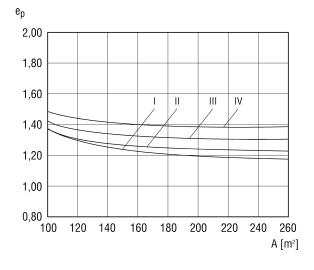
$I - Q_h = 30 \text{ kWh/(m}^2\text{a})$ II -  $Q_h = 40 \text{ kWh/(m}^2\text{a})$ III-  $Q_h = 50 \text{ kWh/(m}^2\text{a})$
