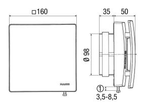
① Screw for adjusting the lamella
