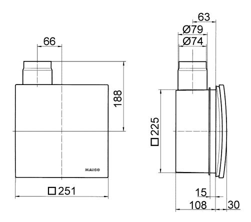
Centro-M / Centro-E / Centro-H exhaust air element with ER-UP/G or ER-UPD recessed-mounted housing
