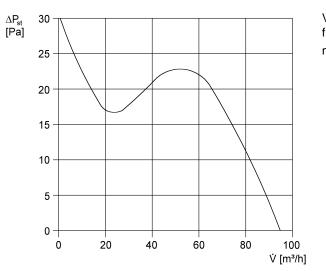
V = 230 or 24 Vf = 50 Hz n = 2650 min<sup>-1</sup>
