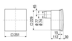
Fan insert ER  $\ldots$  E with ER-UP/GH recess-mounted housing
