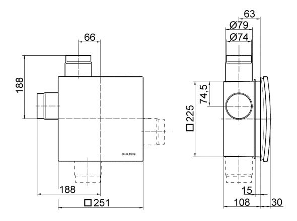
ER fan insert with recessed-mounted housing ER-UP/G or ER-UPD and second room connection
