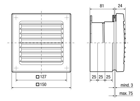
Window cut-out diameter of 115 up to 120 mm
