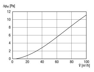
The pressure/air volume characteristic curve shown applies to the clean filter medium. High pressure losses may arise with dirty filters depending on the type and scope of contamination.
