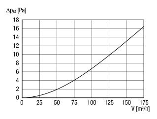
The pressure/air volume characteristic curve shown applies to the clean filter medium. High pressure losses may arise with dirty filters depending on the type and scope of contamination.
