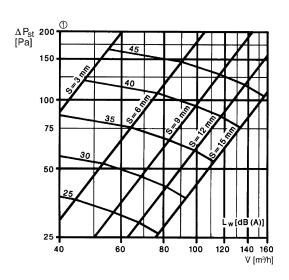
① Valve cone position, S = gap width
