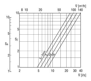
$sec._A$  - Blow out distance in m  $sec._Z$  - Zone length in m s = gap width **PRODUCT**DATA SHEET
