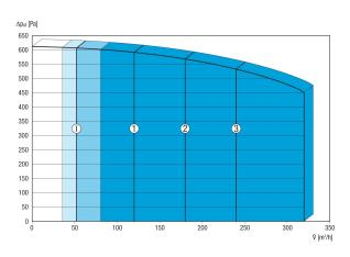
The figures shown indicate the preset ventilation levels ("factory settings").
