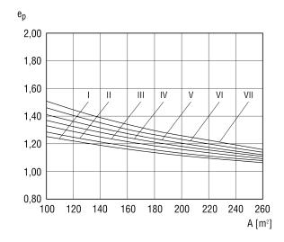
$$\begin{split} I - Q_h &= 30 \text{ kWh/(m}^2 a) \\ II - Q_h &= 40 \text{ kWh/(m}^2 a) \\ III - Q_h &= 50 \text{ kWh/(m}^2 a) \\ IV - Q_h &= 60 \text{ kWh/(m}^2 a) \\ V - Q_h &= 70 \text{ kWh/(m}^2 a) \\ VI - Q_h &= 80 \text{ kWh/(m}^2 a) \\ VII - Q_h &= 90 \text{ kWh/(m}^2 a) \end{split}$$
