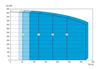
The figures shown indicate the preset ventilation levels ("factory settings").
