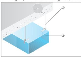
① Ventilation channel, to be supplied by the customer
