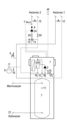
As standard, the AWP is equipped to control a second heating circuit with another forward flow temperature. The second heating circuit must be equipped by the customer with a mixer servomotor and a circulation pump.
