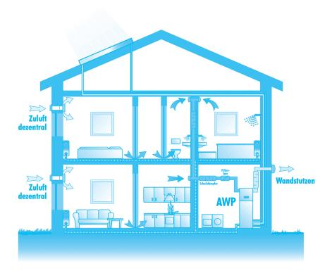
In the case of very low outside temperatures or a very high heat requirement, the exhaust air heat pump covers the residual heat requirement of the heating system using a built-in auxiliary electric heater (electrical re-heating).
