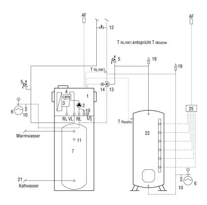
The AWP can be combined with a buffer battery. This permits the use of both inexpensive nighttime power and other sources of power. The discharge control is integrated in the AWP.
