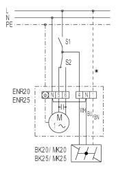
S1 - On / Off S2 - Switching between air extraction and ventilation Terminal 5 - Air extraction Terminal 6 - Ventilation \* - duct only for MK... shutter
