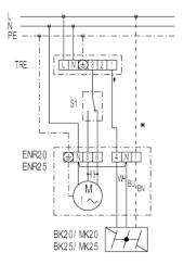
TRE - 5-step transformer (on/off, 5-speed) S1 - Reversing switch (air extraction or ventilation) \* - duct only for MK... shutter BK 20
