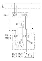
TRE - 5-step transformer (on/off, 5-speed) S1 - Reversing switch (air extraction or ventilation) \* - duct only for MK... shutter BK 31
