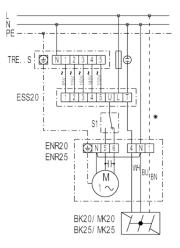
TRE - 5-step transformer, control cabinet installation ESS 20 - 5-step switch (on/off, 5-speed) S1 - Reversing switch (air extraction or ventilation) \* - duct only for MK... shutter
