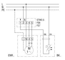
FS6 - Step switch: 2 speeds, ventilation / air extraction (FS 6 cannot be used for ENR 31) FS7 - Step switch: Ventilation / air extraction
