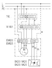
FS6 - Step switch: 2 speeds, ventilation / air extraction (FS 6 cannot be used for ENR 31)
