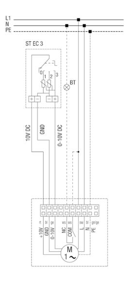
Fuse and main switch provided by customer Levels 1 - 3 up to 7 V DC Levels 2 - 5 up to 9 V DC Level 3 - 10 V DC
