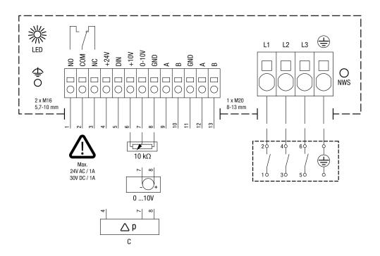
C - Controller NWS - Network screw, max. 0.8 Nm, do not remove
