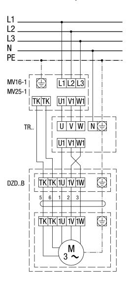
Left-hand operation (air extraction) = standard For right-hand operation, swap 2 phases on fan connection.
