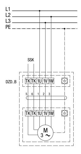
1 speed SSK - control circuit For right-hand operation, swap 2 phases on fan connection.
