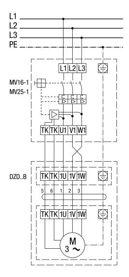
Left-hand operation (air extraction) = standard For right-hand operation, swap 2 phases on fan connection.
