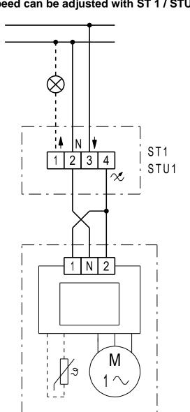
Speed can be adjusted with ST 1 / STU 1
