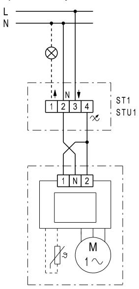
ST 1 speed controller, surface-mounted STU 1 speed controller, recess-mounted
