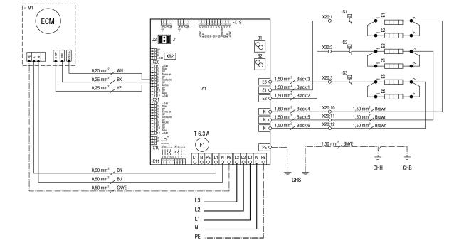
M1 supply air fan J1 Termination BDT J2 Termination Modbus B1 Filter monitoring of supply air B2 Volumetric flow of supply air GHS housing Switch box GHH housing Heating GHB housing Box Power supply / 400V / 3- / N / 50Hz Fuse, external 16A
