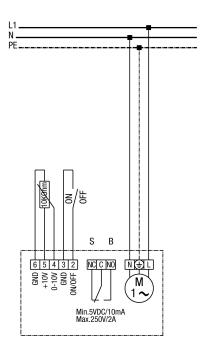
S - fault B - operation Min. 5 V DC / 10 mA Max. 250 V / 2 A
