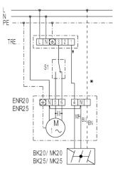
TRE - 5-step transformer (on/off, 5-speed) S1 - Reversing switch (air extraction or ventilation) \* - duct only for MK... shutter
