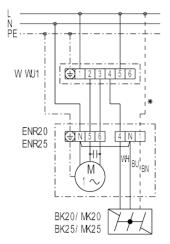
W 1 - Reversing switch (air extraction or ventilation), surface-mounted WU 1 - Reversing switch (air extraction or ventilation), recessed-mounted \* - duct only for MK... shutter
