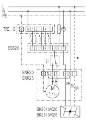
TRE - 5-step transformer, control cabinet installation ESS 20 - 5-step switch (on/off, 5-speed) S1 - Reversing switch (air extraction or ventilation) \* - duct only for MK... shutter
