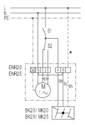
S1 - On / Off S2 - Switching between air extraction and ventilation Terminal 5 - Air extraction Terminal 6 - Ventilation \* - duct only for MK... shutter
