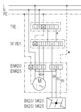
TRE - 5-step transformer (on/off, 5-speed) W 1 - Reversing switch (air extraction or ventilation), surface-mounted WU 1 - Reversing switch (air extraction or ventilation), recessed-mounted \* - duct only for MK... shutter
