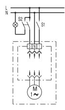
S1 = Base load (low speed) S2 = Full load (high speed)
