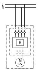
The fan always runs at the base load. If the humidity is higher than the switch-on humidity, the fan will automatically switch to full load.
