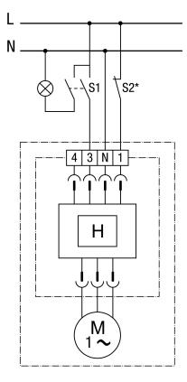
The fan is manually switched on and off with switch S1. The fan always overruns until the air humidity in the room has fallen below the switch-off humidity level.
