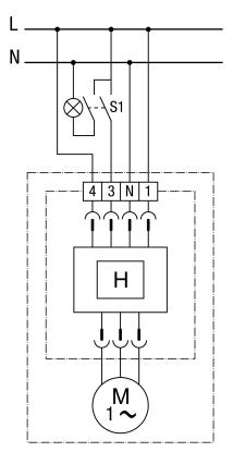
Fan always runs at base load. If humidity is higher than the switch-on humidity, the fan will automatically switch to full load. Additionally, it is possible to manually switch to full load with S1 switch. Using a 1-pin switch can cause reverse polarity voltages. Combination with an X2 capacitor necessary!
