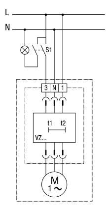
S1 on (after approx. 50 s) S1 off (overrun time 6 min.) Using a 1-pin switch can cause reverse polarity voltages. Combination with an X2 capacitor necessary!
