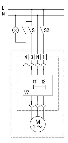
S1 and S2 on (after aprox. 50 s) S1 off (overrun time 6 min.) In addition, the fan can be switched off with switch S2 independent of the room lighting. Using a 1-pin switch can cause reverse polarity voltages. Combination with an X2 capacitor necessary!
