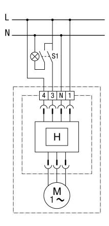
Fan always runs at base load. If humidity is higher than the switch-on humidity, the fan will automatically switch to full load. Additionally, it is possible to manually switch to full load with S1 switch.
