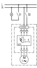
S1 On (after approx. 50 s) In addition, the fan can be switched off by switch S2 independent of the room lighting.
