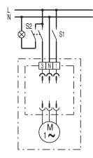
S1 = Base load (low speed) S2 = Full load (high speed)
