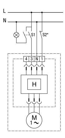
The fan is manually switched on and off with switch S1. The fan always overruns until the air humidity in the room has fallen below the switch-off humidity level.
