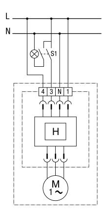
Fan always runs at base load. If humidity is higher than the switch-on humidity, the fan will automatically switch to full load. Additionally, it is possible to manually switch to full load with S1 switch.
