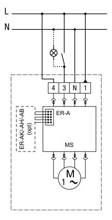
opt - optional MS - motor control Full load can be switched with permanent base load Connection is made in the housing
