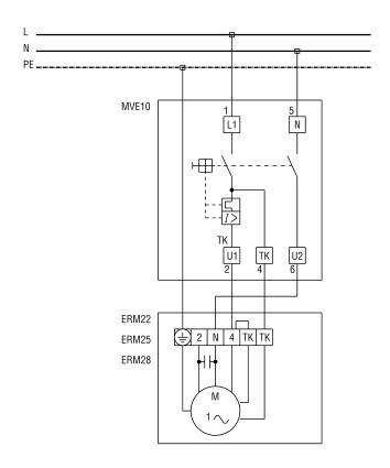
MV 10 motor protection switch, to be supplied by the customer
