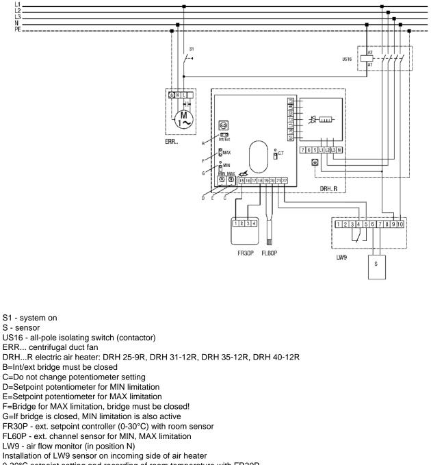
0-30°C setpoint setting and recording of room temperature with FR30P
