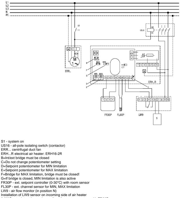
0-30°C setpoint setting and recording of room temperature with FR30P
