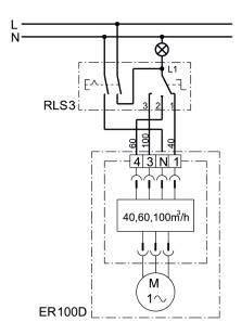
RLS 3 - Room air control with zero position and switch for room lighting
