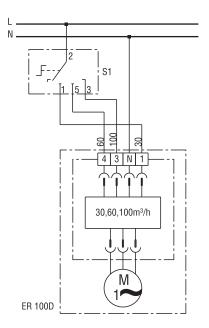
S1 Three-step switch DS 3N with zero position
