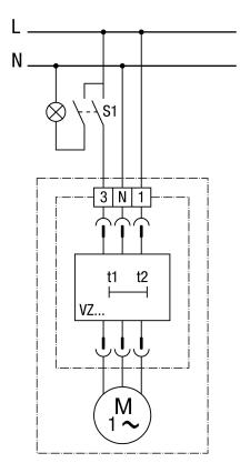
S1 on (after aprox. 50 s) S1 off (overrun time 15 min.) Using a 1-pin switch can cause reverse polarity voltages. Combination with an X2 capacitor necessary!
