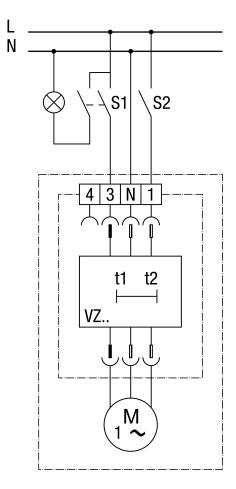
S1 and S2 on (after aprox. 50 s) S1 off (overrun time 15 min.) In addition, the fan can be switched off with switch S2 independent of the room lighting. Using a 1-pin switch can cause reverse polarity voltages. Combination with an X2 capacitor necessary!
