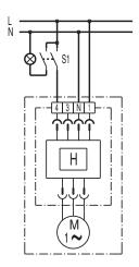
The fan is switched manually to base load with switch S1. If humidity is higher than the switch-on humidity, the fan will automatically switch to full load.
