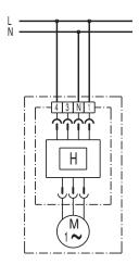
Fan always runs at base load. If humidity is higher than the switch-on humidity, the fan will automatically switch to full load.
