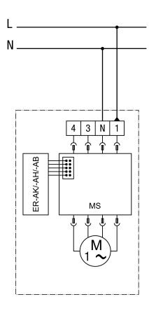
MS - motor control Connection is made in the housing
