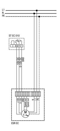
Fuse and main switch provided by customer Switching the ventilation box on and off only via 0-10 volts
