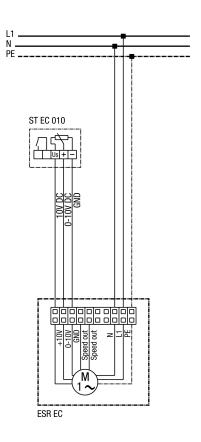
Fuse and main switch provided by customer Switching the ventilation box on and off only via 0-10 volts
