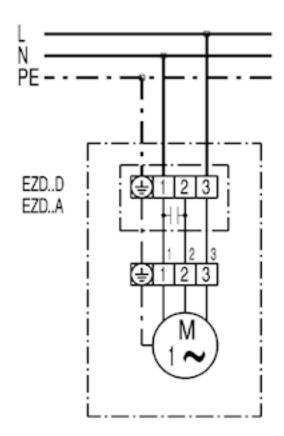
Right-hand rotation: EZD 25/2 A with air blown across the motor
