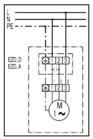
Right-hand rotation: EZD...D with air blown across the motor
