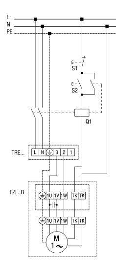
S1 - Off switch S2 - On switch Q1 - US 16 T contactor
