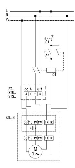
S1 - Off switch S2 - On switch Q1 - US 16 T contactor
