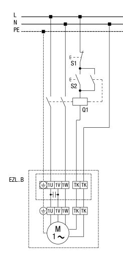
S1 - Off switch S2 - On switch Q1 - US 16 T contactor
