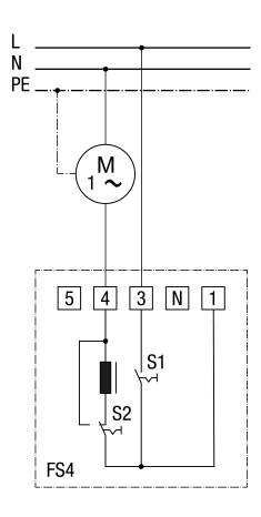
FS 4 step switch S1 switch: On / Off S2 switch: fast/slow M1 fan motor
