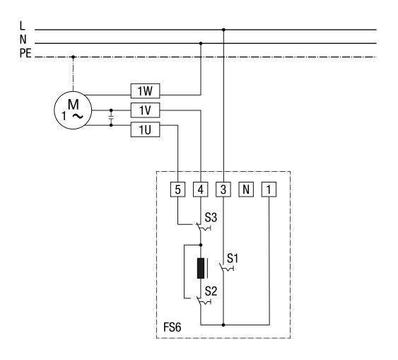
FS6 step switch S1 switch: On / Off S2 switch: fast/slow
