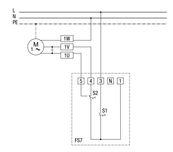
FS7 step switch S1 switch: On / Off S2 switch: Rotational direction (air extraction / ventilation) M1 fan (capacitor motor)
